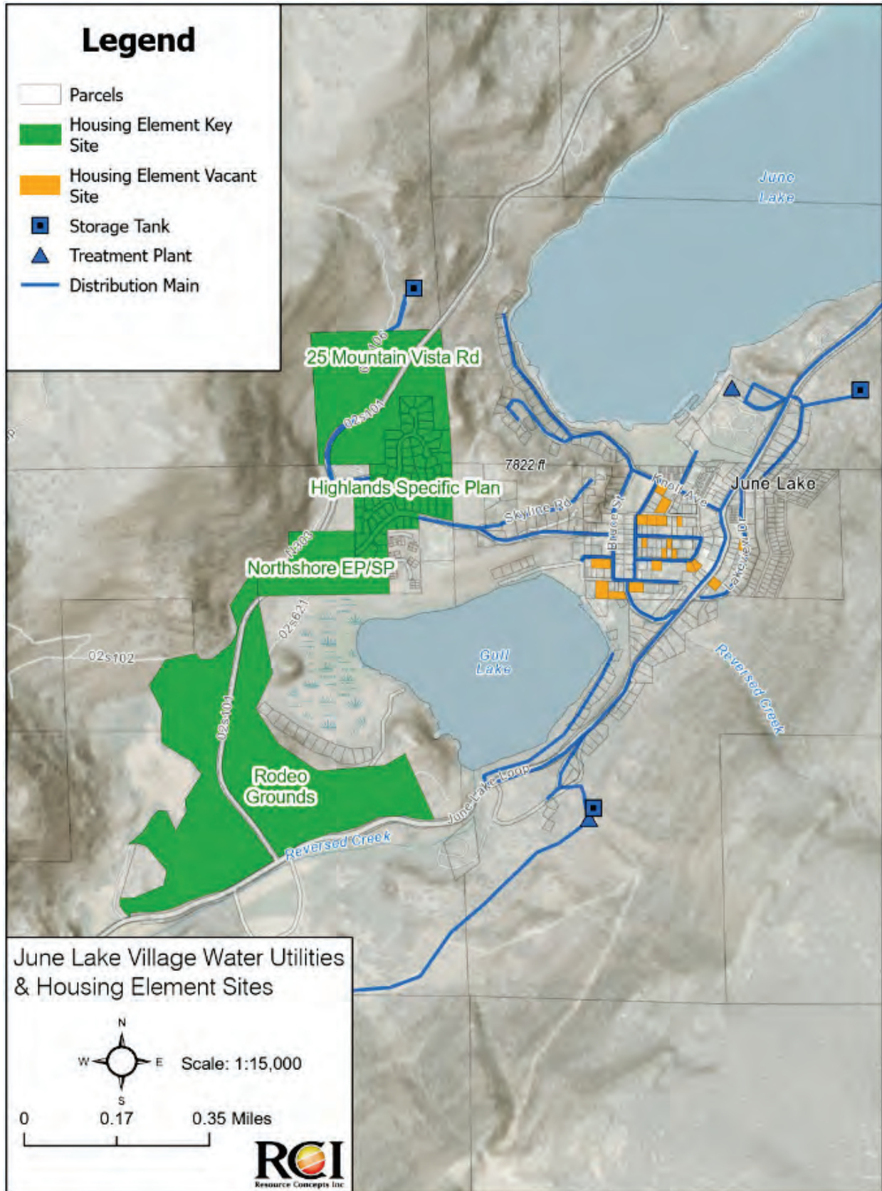
Figure 2: June Lake PUD Village Water System
